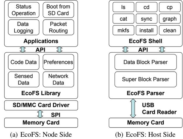
Figure 6. The block diagrams of EcoFS.
