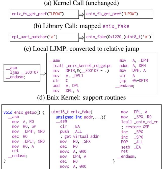
**Figure 4. (a)-(c): Transformation and (d) support for position independent code.**
