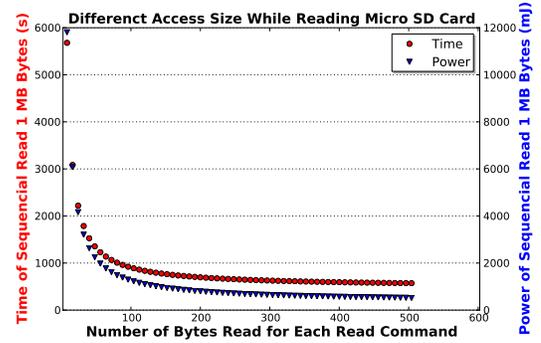
**Figure 10. SD card reading using different block lengths.**
