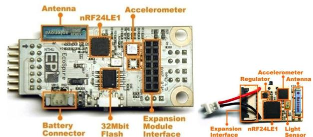
Figure 8. (a) EcoSpire node:  $23 \times 50 \text{ mm}^2$ ; (b) EcoSpire simple node,  $13 \times 20 \text{ mm}^2$ .
