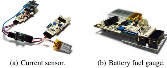
(a) Current sensor. (b) Battery fuel gauge.
