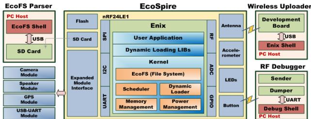
Figure 2. The block diagram of Enix.
